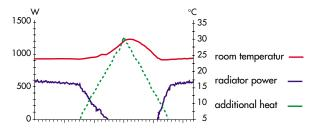
Thermostat switches off at 1°C of increase.
